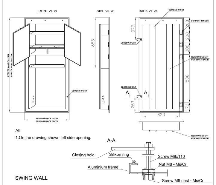
Metal swing wall is a part of the sanitary cabins equipment. It is mount to the wall of sanitary cabin by hinges and performs a function of locker and a mirror.
